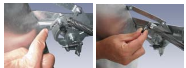
Fig 12: Subsequent alteration of discharge angle in increments of 5^\circ (up to 20^\circ in total)
