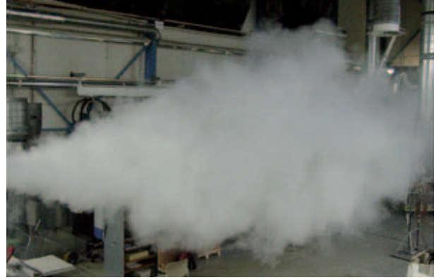
Fig. 4: Jet dispersion with twist nozzle
