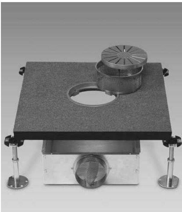
Figure 7: Floor displacement outlet Q-B-DN 200, installation example: Perforated sheet metal distributor basket VPD with throttle device and floor tile with clamp insert in a through bore; below it connection box for duct connection
