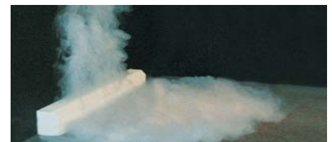
Air jet pattern of Q-SH (when heating)
