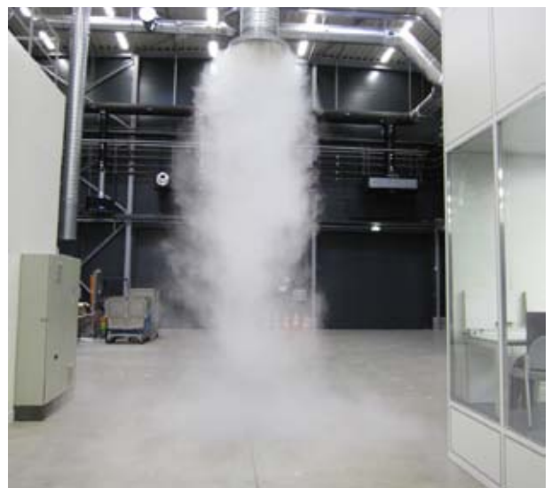
Fig. 6: Vertical discharge from a great height, jet pattern made visible by smoke tracer
